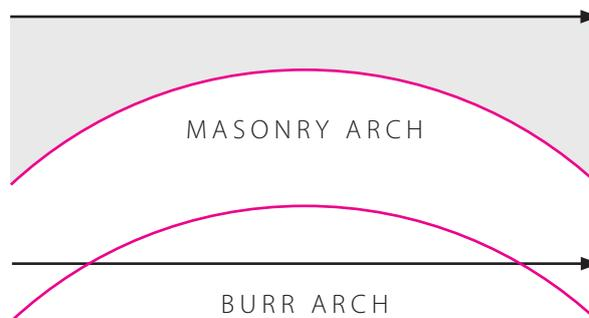
Drawing 8 shows the road surfaces as black lines, the arches as magenta lines and their relationship in masonry and timber bridges.
