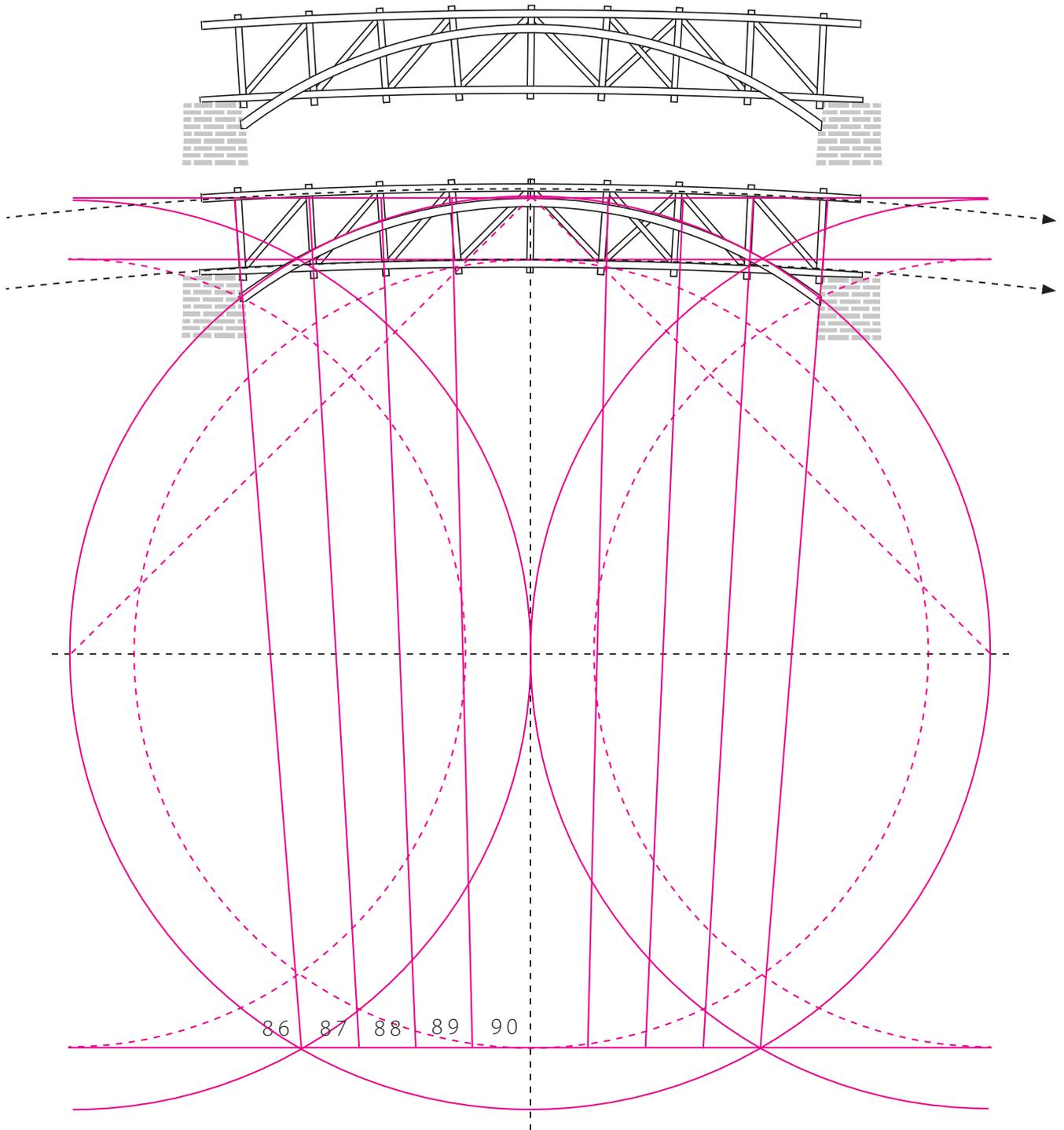
Drawing 7 is doubled in scale with the bridge superimposed on the geometrical construction so that the intimacy of the two is clear. The bridge is also shown separately for comparison. It can be seen that the masonry buttressing at either side of the bridge follows the angles of the outer king posts and that the bracing in the centre of the bridge connects the main circle's W and E poles to its N pole.
