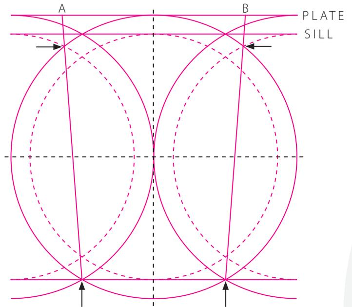
Drawing 5 shows the plate line AB and foot line CD each divided into eight equal sectors which are linked to form king post angles between the plate and sill.
